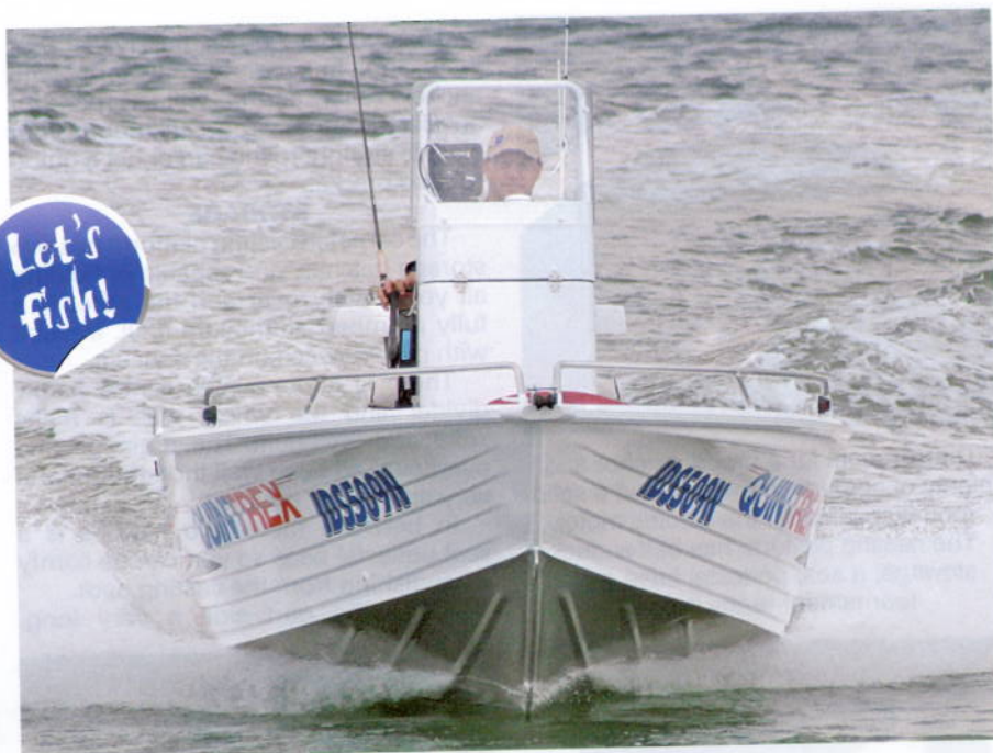
The Millennium Hull and Quintrex Flared Bow afford stability at rest, quick planing and a soft, dry ride.
